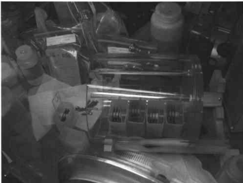
Figure 3-2 Partially loaded sample chamber inside the anoxic glove box. A second row of brine containers will be placed into the chamber and then the humid atmosphere replicates will be hung at the end of the chamber.
